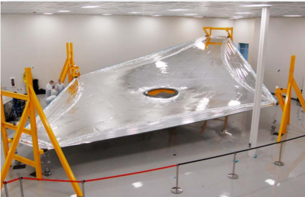
Figure 4: Template layer 3 mounted on the shape test fixture at Mantech. The membrane is tensioned via four catenary cables. The purpose of the test is to measure the three-dimensional shape of the membrane.
