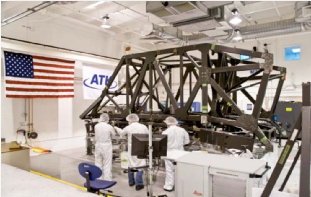
Figure 2: Center Section Integrated to the Backplane Support Frame (CS/BSF)
