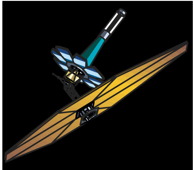
An early concept for the James Webb Space Telescope – known at the time as the Next Generation Space Telescope – was designed by a Goddard Space Flight Center-led team. It already incorporated a segmented mirror, an “open” design, and a large deployable sunshield.
